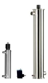
The UV reactor is totally in stainless steel AISI 304 or 316L <u>internally/externally polished</u>; the stainless steel of its chemical/physical characteristics is particularly suitable for the treatment of primary waters, and being polished also in the internal part it is completely without porosity that could favour the keeping of spores; moreover, being glass polished, the germicidal action of the lamps is increased.
