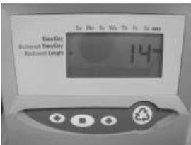
The back wash time will be pre-set but may need altering to suit your requirements. To amend this setting press the set button to start the display flashing, then alter the figure using the up and down arrows, then press the set button to confirm the setting.
