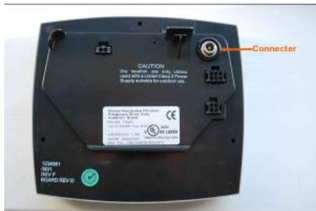
All valves are low voltage valves with a 240V transformer. With the power off connect the transformer provided to 240V supply. With the power OFF plug the flying lead into the connector on the controller (Fig A.9). If you have an in line transformer this need to be wired into a fused switch.
