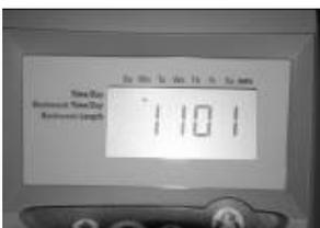
Press the set button. The TIME should now be flashing, use the up and down arrows to set the correct time of day (24hrs format). Once the correct time has been selected, press the set button to confirm. The following will then be displayed.
