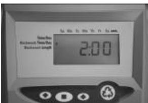
This normally defaults to 2.00am but can easily be changed to a more suitable time if required by pressing the square set button to start the display flashing, adjusting the time using the up and down arrows then press the square set button to confirm. The following will then be displayed.
