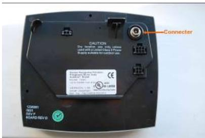
All valves are low voltage valves with a 240V transformer. With the power off connect the transformer provided to 240V supply. With the power OFF plug the flying lead into the connector on the controller (Fig A.11). If you have an in line transformer this needs to be wired into a fused switch. Ensure that the flying lead cannot get caught on the camshaft or any of the valves moving parts.
